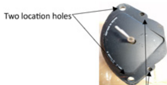
Two location holes Two screws holding the clock face to the mechanism.
