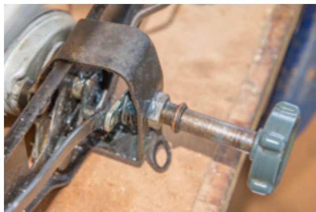
Below - the motor now mounted on its two bushes on and against the wiper mechanism. Note the grey hand wheel referred to later.
