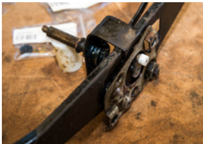
Left - the round bar going off to the left is the part that projects into the cabin and on it is fitted a grey hand wheel..
