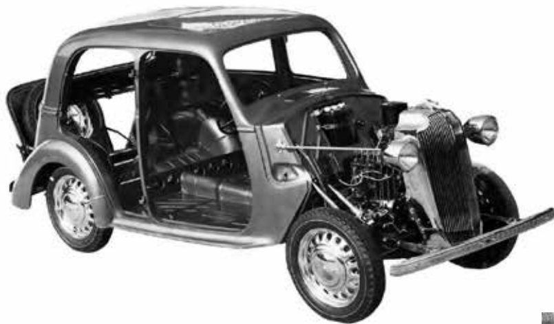
Fig 4, Vauxhall Ten welded body
